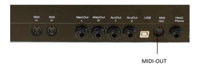
The Midi-Out can be used to connect a sound module or synthesizer which then can be played together with the organ sound of the X3. This way the X3 can be used as a velocity sensitive controller keyboard.
