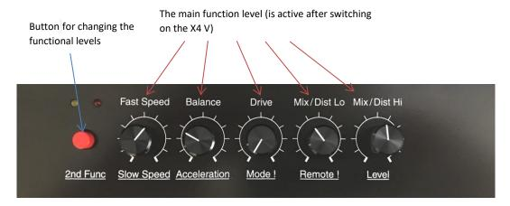
**Fast Speed:** The Fast Speed knob adjusts the bass and treble rotors' speeds while the unit is in FAST mode. Twist the knob to the
