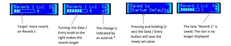
Press the Data Entry knob for 2 seconds to permanently store parameter changes. The asterisk disappears after saving.
