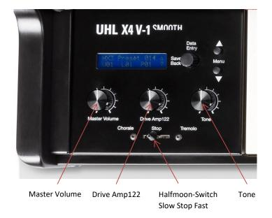
**Master Volume:** If, for example, the overdrive control "Drive Amp122" is turned up, the overall level becomes considerably louder. This can also lead to the override of the Vent II. In this case, the "Overload-Led" lights up. This too high level must then be adjusted with the master volume control (turn to the left).
