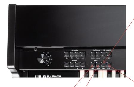
Sep. (Separate bass): The pedal bass is always separately available at the "Separate Bass" output socket on the back of the organ.
