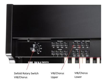
Rotary switch is used for selecting one of the six effects vibrato V1, V2, V3 or chorus C1, C2, C3. The two push-buttons Vib/Chorus Upper and Lower are used to switch the effect on/off, either for the upper or lower manual. Ex-factory the Vib/Chorus parameters are set according to a real vintage organ. All Vib/Chorus parameters are programmable in the Menu/Display panel (see page 27).
