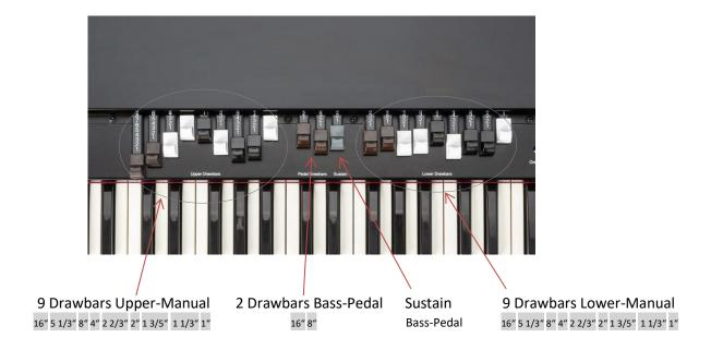
The X4 V organ has 2 sets of nine drawbars, one for the upper manual and one for the lower manual plus 2 drawbars for the bass pedal. A third bass pedal drawbar controls sustain of the bass sound. The drawbars are used for adjusting the basic harmonics of the X4 V. This offers a wealth of sound shaping options. All 9 drawbars pulled out results in 9 different harmonic tones per key.
