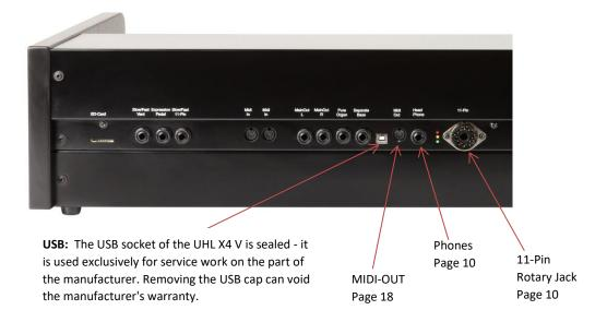
**USB:** The USB socket of the UHL X4 V is sealed - it is used exclusively for service work on the part of the manufacturer. Removing the USB cap can void the manufacturer's warranty.
