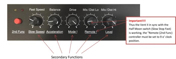
**Slow Speed (2nd Func):** The Slow Speed knob adjusts the bass and treble rotors'speeds while the unit is in SLOW mode. Twist the knob to the
